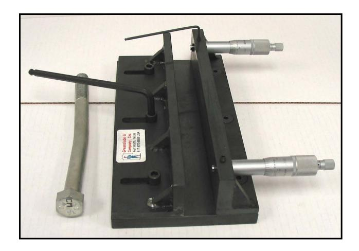
This gage is used to inspect for the straightness or camber in a bolt or screw. The allowance for bend or camber is specified in the various product standards.
